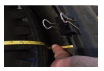
Make sure the tape is in contact with the tire all the way around the inside and take the measurement at the opposite edge of the inside of the tire.
