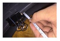
Secure one end of the measuring tape to the edge of the inside of the tire.
